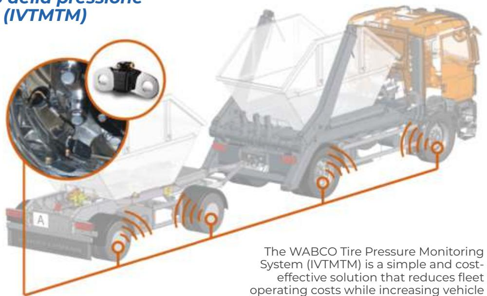
The WABCO Tire Pressure Monitoring System (IVTMTM) is a simple and cost-effective solution that reduces fleet operating costs while increasing vehicle safety. The driver is informed about the tire pressure of all monitored wheels during driving.
